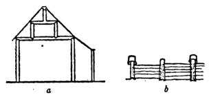
Fig. 2. a. Skeleton framework at end of building showing how weight is carried by pillars and beams, and how roof may be extended to form verandah. b. Sketch of fence.
